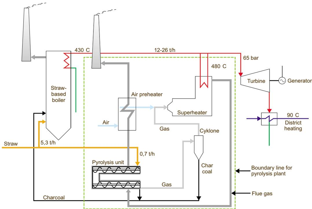
Figure 23: Simplified diagram of the pyrolysis plant at Haslev Kraft-varmeværk (CHP plant).
