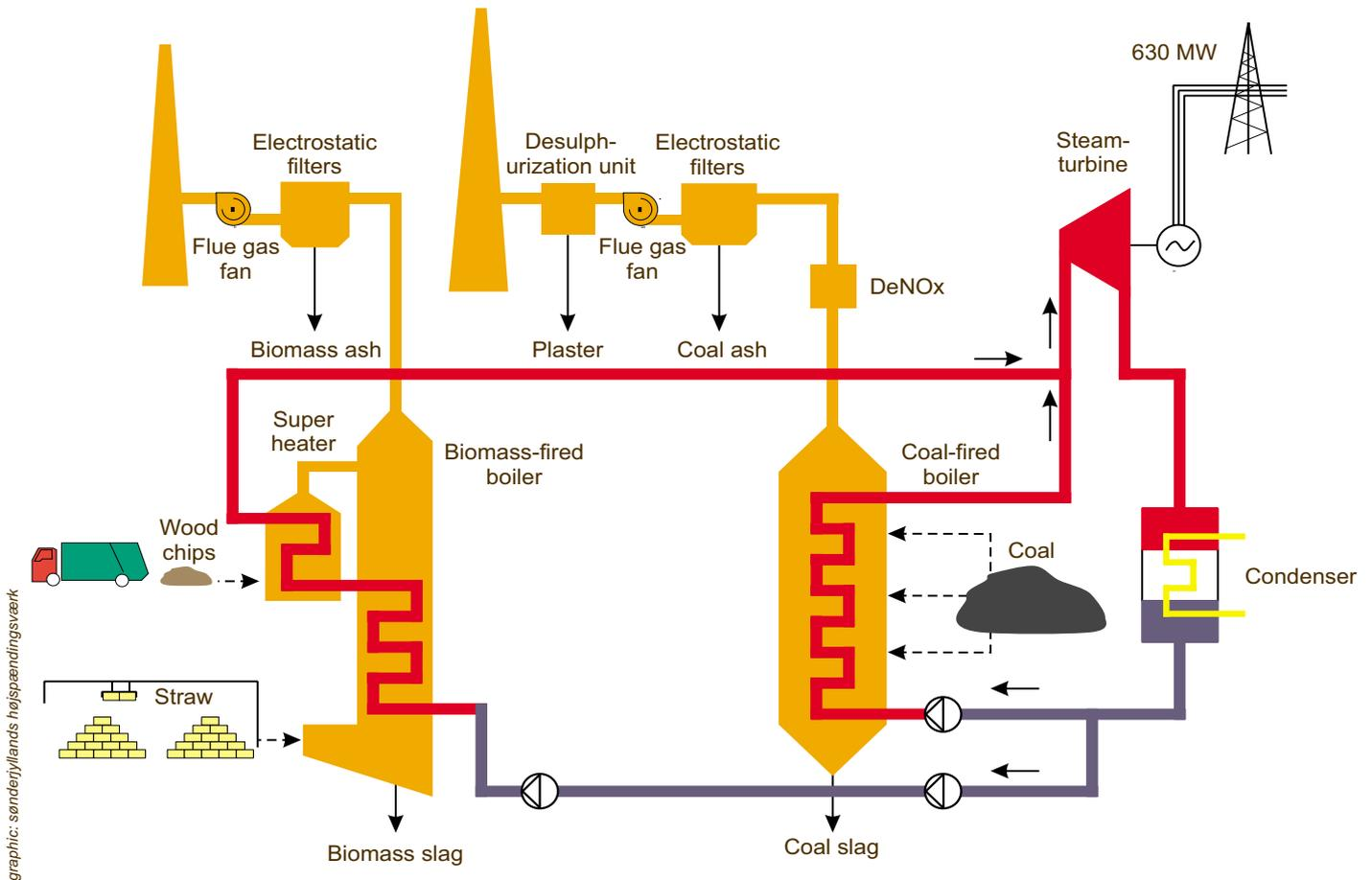
Figure 22: Simplified diagram of Enstedværket's biomass-fired boiler of 40 MW electrical power and the coal-fired boiler of 630 MW electrical power. The biomass-fired boiler substitutes the use of the 80,000 tonnes of coal/year, thereby reducing the amount of CO<sub>2</sub> being released to the atmosphere by 192,000 tonnes/year.
