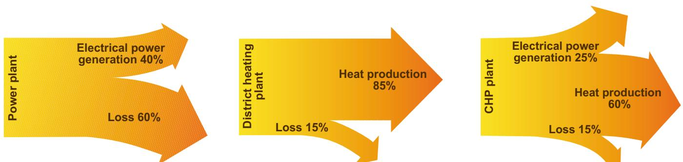
Figure 20: By separate electrical power generation and heat production at a power plant and a district heating plant, the losses are much larger than by combined heat and power production at a CHP plant. Losses include own consumption at the plant
