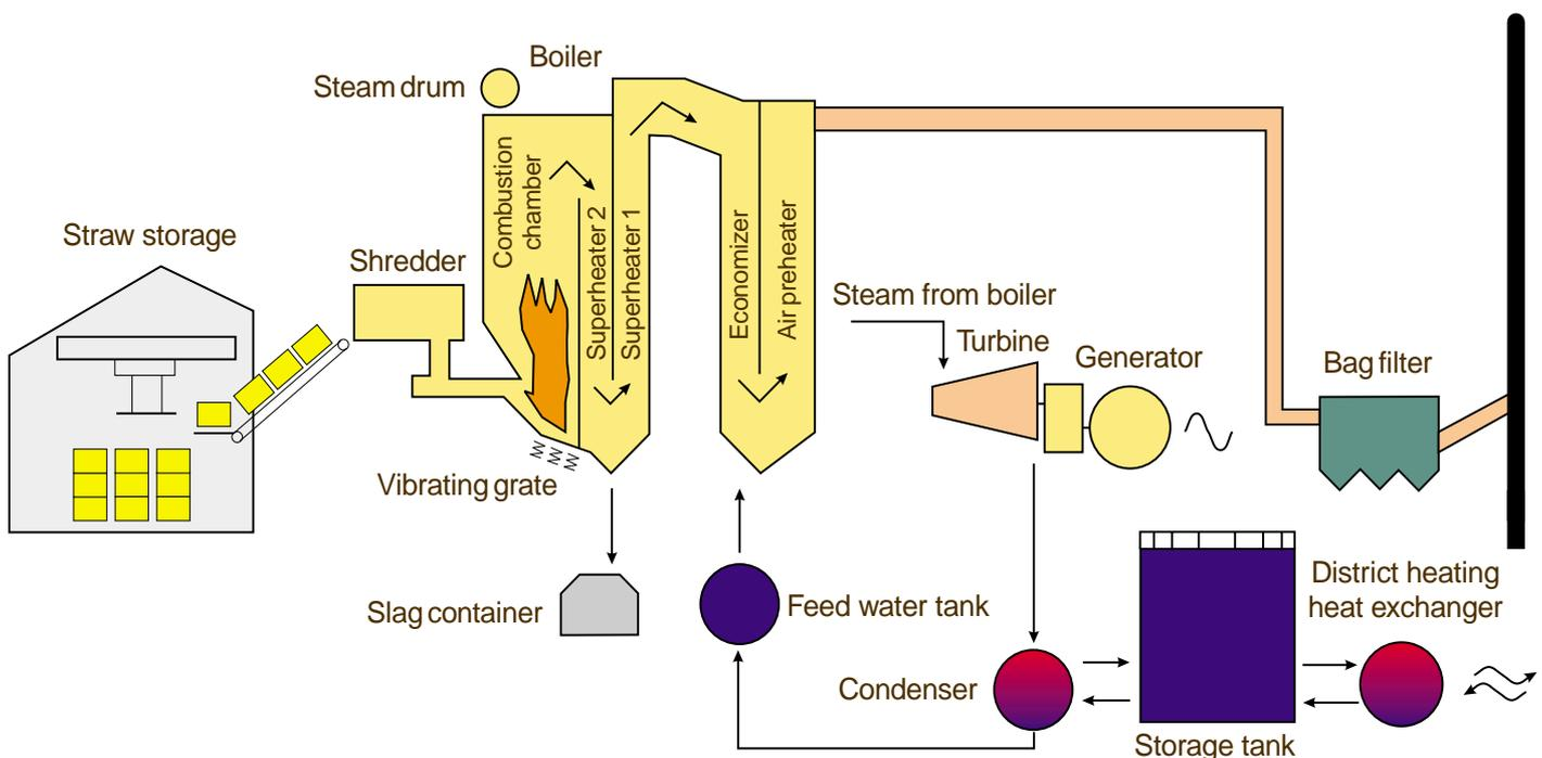
Figure 21. Simplified diagram of Rudkøbing Kraftvarmeværk (CHP plant). The flue gas passes through the combustion chamber to the superheater section and further through an economiser and air preheater and is cleaned in a bag filter before being released through the chimney at 110°C.
