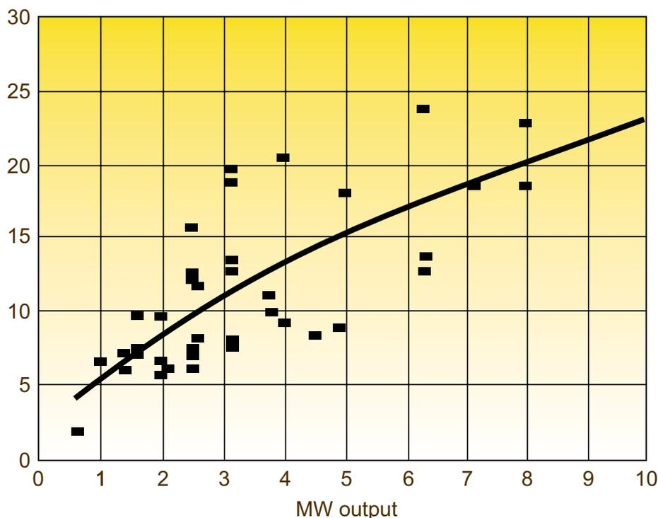
Figure 18: Cost of construction by the million (DKK) per MW installed output, adjusted to the price level of 1995. The price includes site, land development, buildings, installation of machinery, and projecting. The information is based on 40 plants that only use straw. The price spread can be explained by different size of storage, the general quality of the plant, fluctuations of the market in the period from 1983-1995, and that individual plants have included a storage tank in the price.
