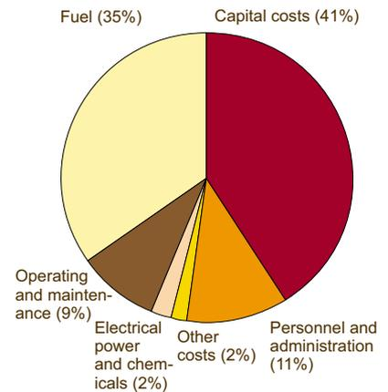
*Figure 19: Distribution of costs in percentages concerning the example illustrated/calculated. The costs in connection with repayment of loan (capital costs) and the purchase of straw and oil make out 76% of the plant's costs.*
