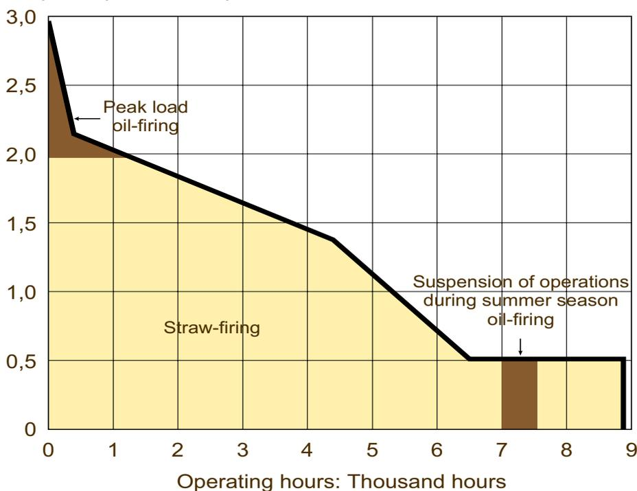
Figure 17: The duration curve for a 3 MW boiler plant with a 2 MW straw-fired boiler. Peak load and stand-by load by a 3 MW oil-fired boiler
