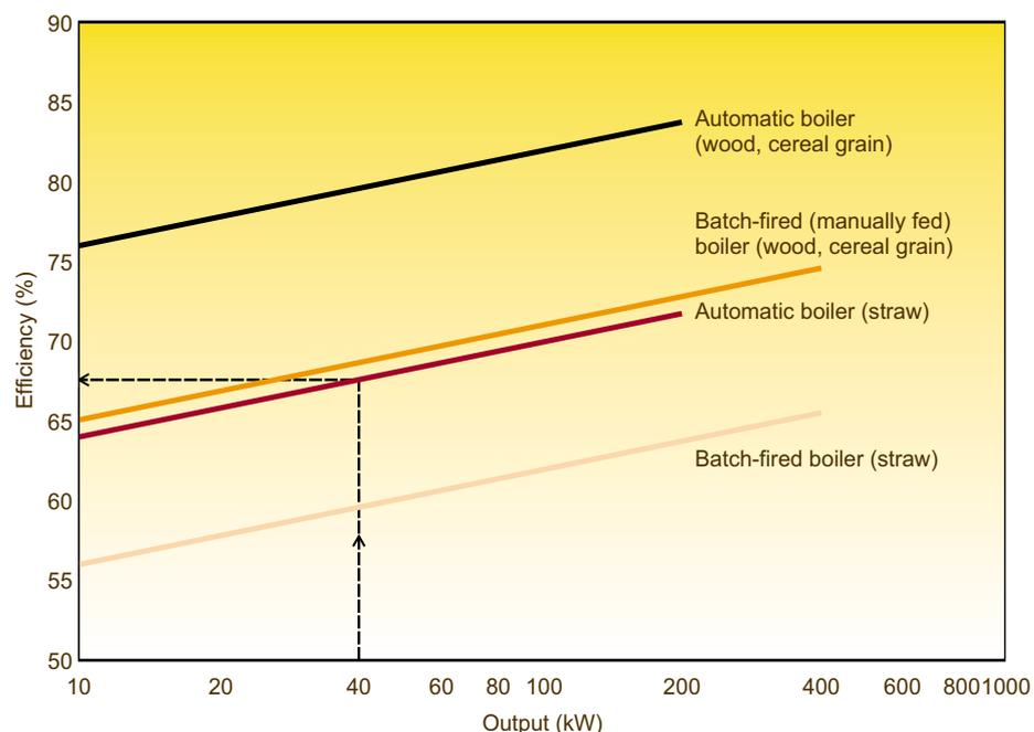
Figure 16: Efficiency minimum values depending on the type of boiler. For an automatic straw-fired boiler of 40 kW to be approved, a minimum efficiency of 67% is required.
