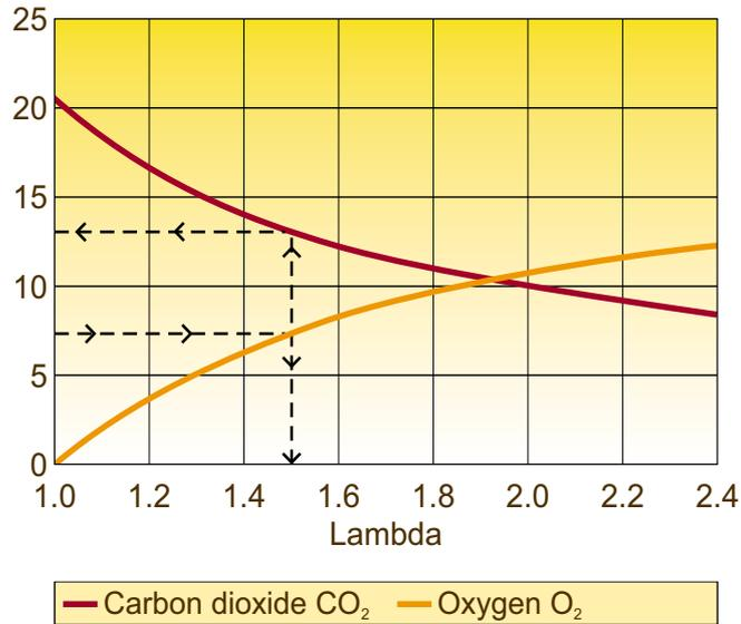
Figure 6: Ideal combustion of straw is performed by excess air of between 1.4 and 1.6. As an example, 7.5% oxygen is measured in the flue gas. The curve illustrates the presence of approx. 13% carbon dioxide with excess air being 1.5%.
