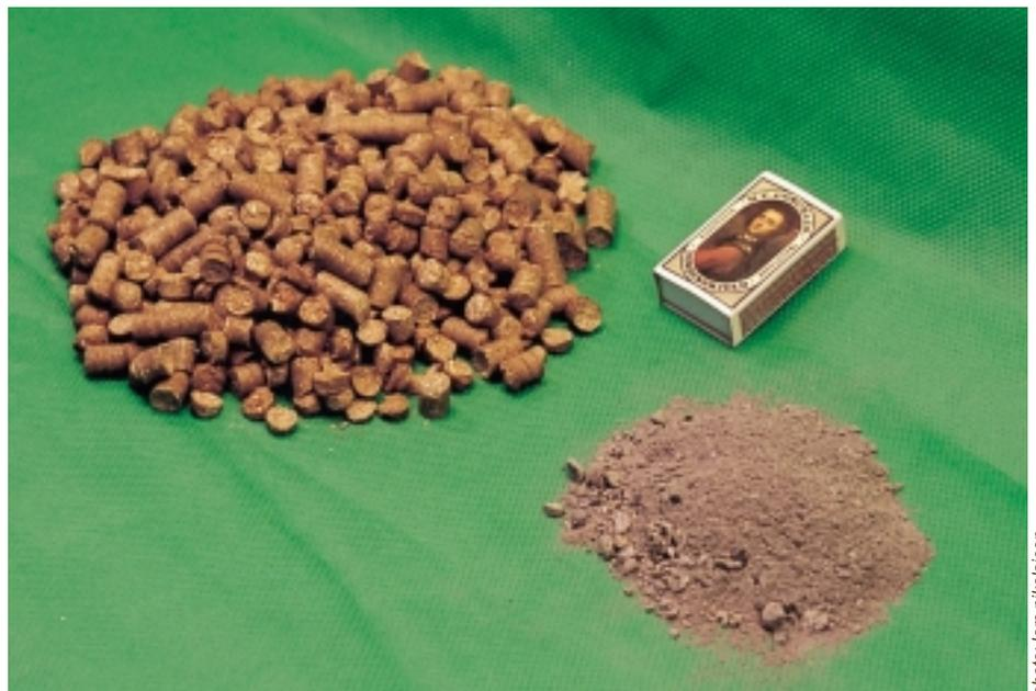
Straw pellets of a diameter of 10 mm mixed with molasses and kaolin and the resulting ash content of 8-10%. Kaolin prevents the ash from forming clinker. Molasses makes the pellets stable during transport
