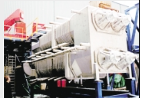
Haslev CHP Straw pyrolysis for more efficient electricity generation
