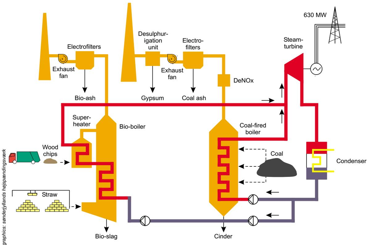
Figure 26: Schematic diagram of Enstedværket's bio-boiler of 40 MW<sub>e</sub> and coal-boiler of 630 MW<sub>e</sub>. The bio-boiler replaces the consumption of 80,000 tonnes of coal per year, thus reducing CO<sub>2</sub> emissions to the atmosphere by 192,000 tonnes per year.
