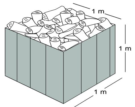
Figure 10: A loose volume cubic metre. For beech and spruce with a moisture content of 20% of the total weight, the solid mass content is 45%. The calorific value of a loose volume cubic metre of beech in 40 cm pieces with a moisture content of 20% is approx. 4.8 GJ.
