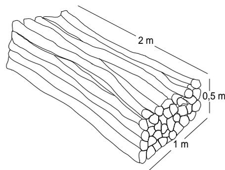
Figure 9: One cubic metre stacked volume of whole-tree wood. A  $\text{m}^3$  stacked volume of beech consisting of 1-meter pieces contains 65% solid mass, while one  $\text{m}^3$  stacked volume of 3-meter pieces contains 55% solid mass. The calorific value of one stacked  $\text{m}^3$  of beech in 2-meter pieces with a moisture content of 20% is approx. 6.5 GJ.
